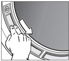
Use your fingers or a vacuum cleaner to remove the fluff from the two fluff filters in the door opening.
